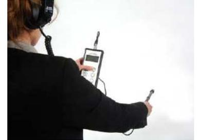
**Portascanner™** ultrasonic hatch cover tester II is an improved version of the Portascanner™, first produced in 1993. The research, development and re-design has been carried out by our in-house team in conjunction with several years' customer surveys and trials, to improve ultrasonic watertight integrity testing as an alternative to water hose or pressure testing. The new model incorporates lightweight materials and state of the art electronics.
